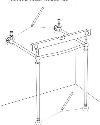
Using a 1/4" drill bit drill the six holes on the marked positions.
